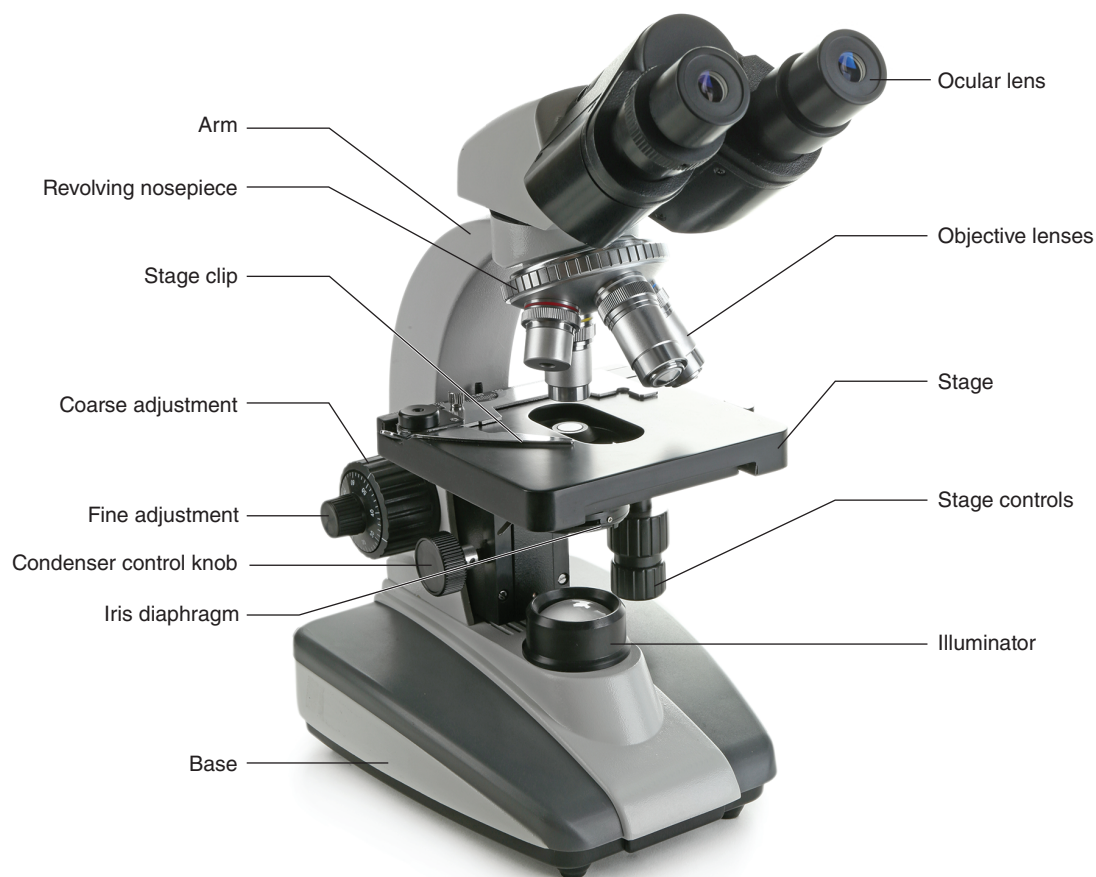
FIGURE 1-1 The parts of a compound light microscope.
