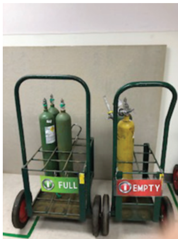
FIGURE 1-18 A portable cylinder cart allows for the cylinder to be safely stored for use during patient transport or ambulation.
