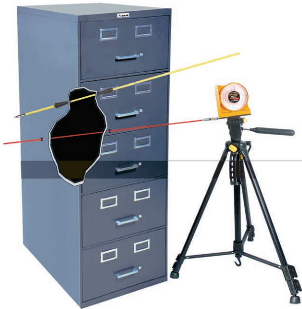
FIGURE 2-9 A laser can be used to determine a bullet's trajectory.
