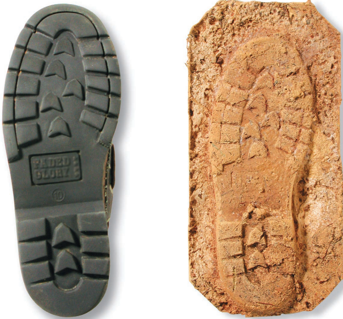
FIGURE 2-8 Molds of shoeprints may be created with silicone rubber.
