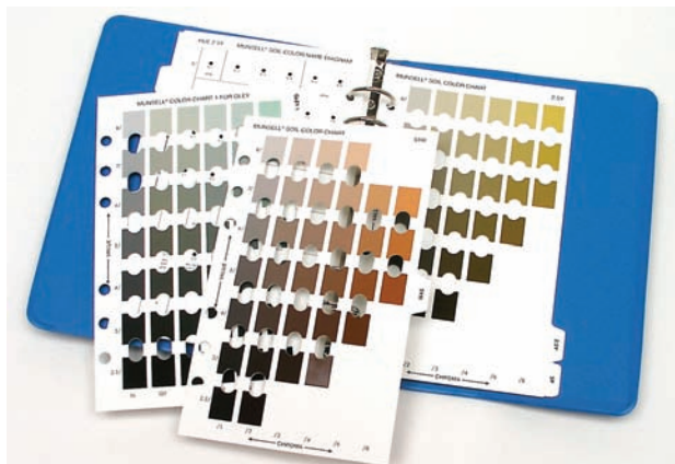
FIGURE 3-6 Soil sample color is described with a Munsell soil color code. The soil is matched to color chips in the manual.
