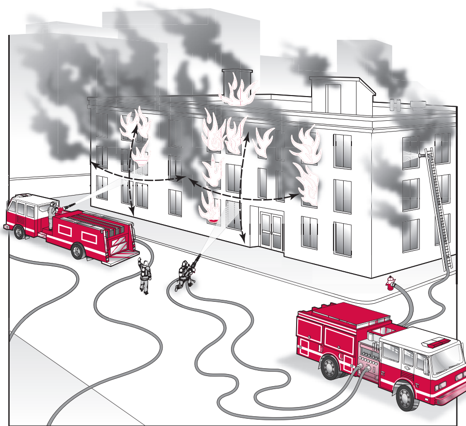
Figure 9-9 Master streams must be moved both vertically and horizontally to cover the entire area involved.
