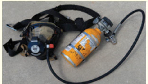
Figure 2-24 A supplied-air respirator may be needed for special rescue operations.
