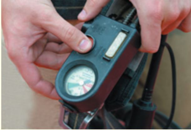
Figure 2-28 A PASS device can be integrated into an SCBA.
