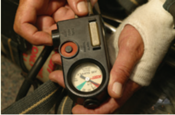
Figure 2-19 A PASS device can save a fire fighter's life.
