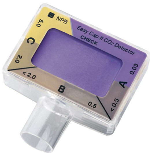
FIGURE 2-15 Colorimetric \text{CO}_2 sensor designed to confirm endotracheal intubation. It fits between the endotracheal tube and the manual bag-valve- \text{O}_2 device.
