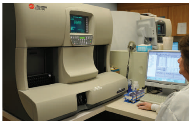
Figure 1-10. A medical technologist checks CBC results on the Beckman Coulter® LH780 Hematology Analyzer.
