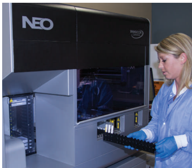
Figure 1-14. NEO Immucor Gamma blood bank automated instrument being loaded with blood samples for type and screen.
