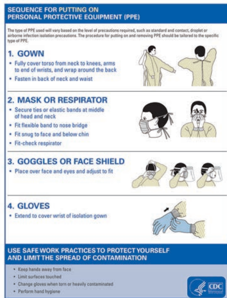
FIGURE D4 The proper sequence of putting on personal protective equipment (PPE).
