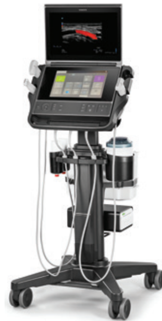
Figure 14-1 SONOSITE PX point-of-care ultrasound system displaying a brachial artery imaged with a high-frequency linear transducer.
